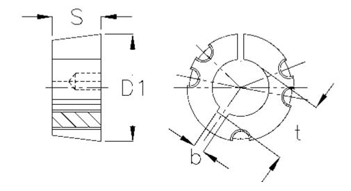
$\begin{array}{lll} b & = 18 \\ Bore & = 65 \\ Bush type & = 4040 \\ D1 & = 146 \\ S & = 101,6 \\ Screw size & = 5/8 \times 1 \ 3/4" \end{array}$
